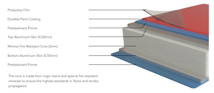
The top coil is coated using a roller coating technique with a 2 or 3 coat, high-performance Kynar / Hylar fluorocarbon (PVDF) coating , FEVE (Lumifon) coating, NANO PVDF or HDPE Coating.
